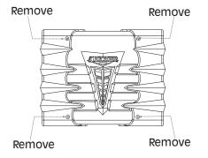
With the shroud removed, drill 4 holes using a 7/64" drill bit and use the supplied #8 screws to mount the amplifier.
